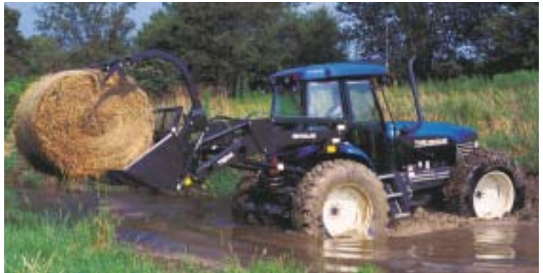
True four-wheel drive with four equal-size tires provides superior traction in wet, icy or muddy conditions.
