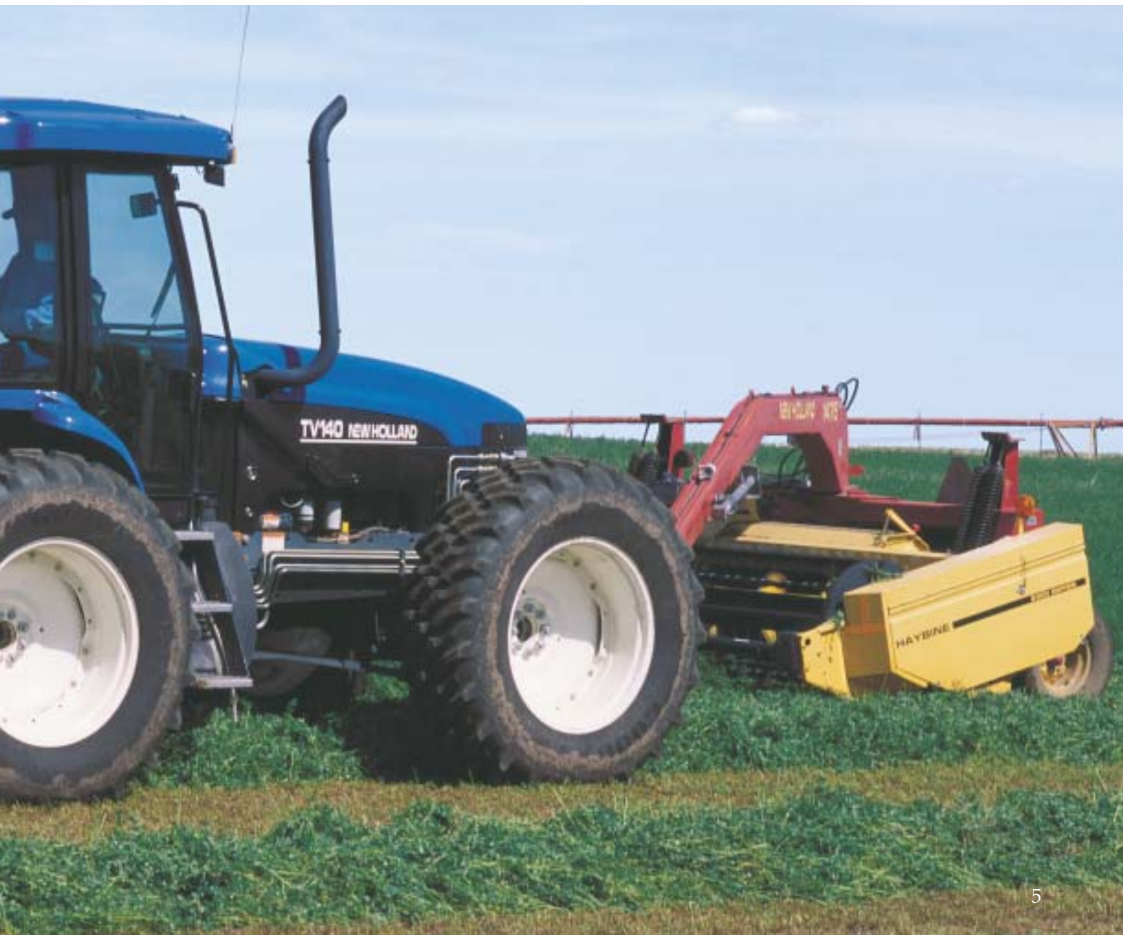
Articulated steering lets you make sharp turns and maneuver in tight areas a typical tractor can't. If one end of the tractor fits, the other end will, too.
