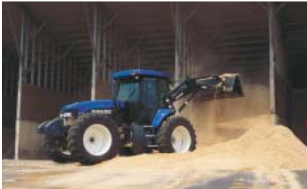
Articulated steering lets you make sharp turns and maneuver in tight areas a typical tractor can't. If one end of the tractor fits, the other end will, too.
